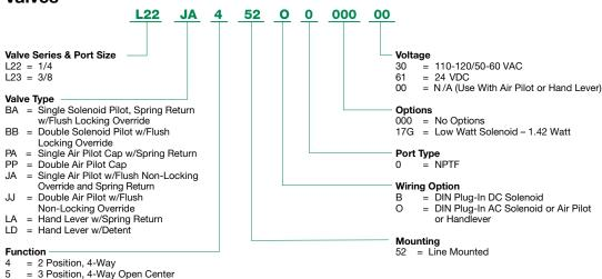
NOTE: Plug connector is NOT included with DIN solenoid. Order plug-in connector assembly separately (see ordering information below).
