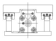
Single chamber bore sizes 25mm to 50mm in extruded aluminum alloy Various supply port configurations available
